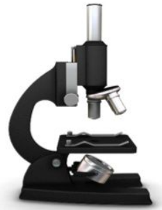
A compound microscope with a single eyepiece and two objective lenses.
